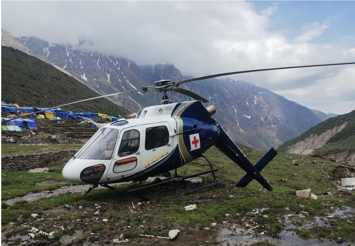
Fig 01: Final resting position of the helicopter with broken tail boom.
